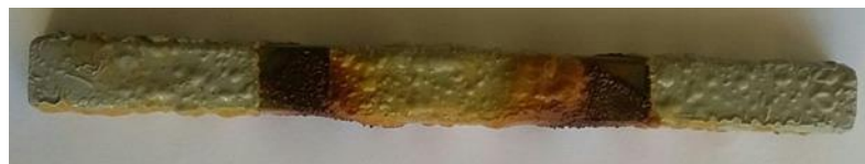
Figure 3-5. Shows corrosion products on the base metal areas of the welded specimens
