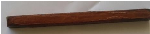
Figure 7. Shows corrosion products on the specimen
