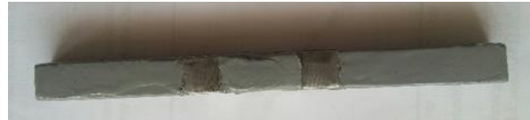
Figure 4. Shows the painted specimen except the heat affected zone area
