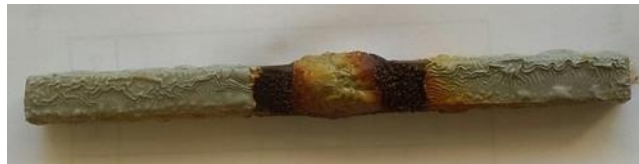
Figure 3-4. Shows corrosion products on the heat affected zone of the welded specimens
