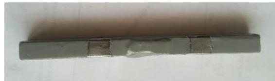
Figure 5. Shows the painted specimen except the base metal area
