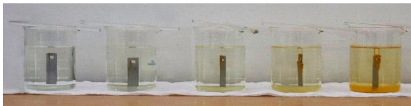
Figure 4 Coupons after 168 hrs. of immersion in 2, 4, 6, 8 and 10 g/L of \text{NaNO}_2 solutions (from right to left)
