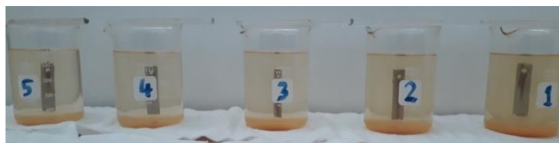
Figure 6 Coupons after 168 hrs. of immersion in 2, 4, 6, 8 and 10 g/L of \text{Na}_2\text{MoO}_4 solutions (from right to left)
