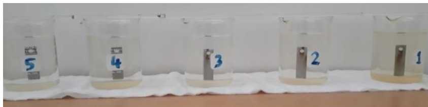
Figure 8 Coupons after 168 hrs. of immersion in 2 g/L of NaNO 2 +2, 4, 6, 8 and 10 g/L of Na 2 MoO 4 solutions (from right to left)
