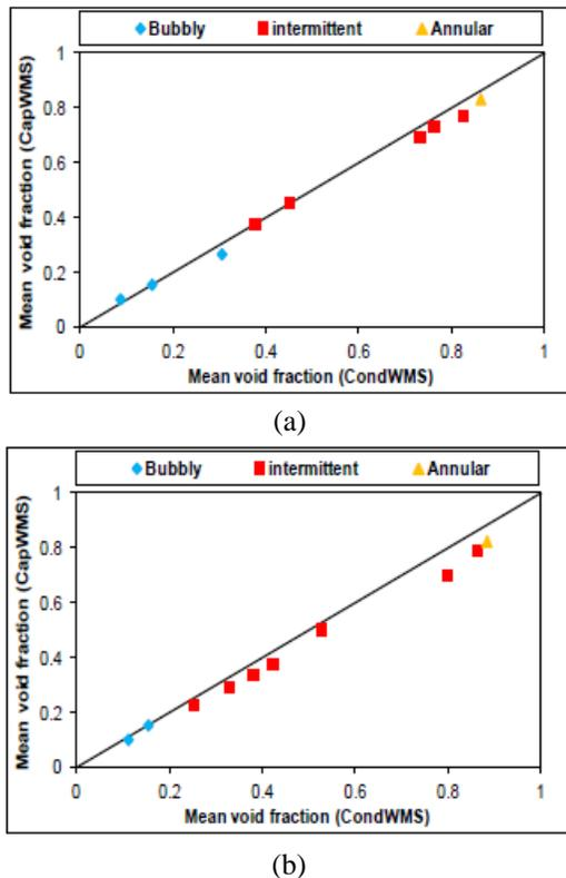
Figure 4: shows the void fraction and the flow regimes extracted from the CondWMS and CapWMS at (a) the lower downward section and (b) the higher upward section
