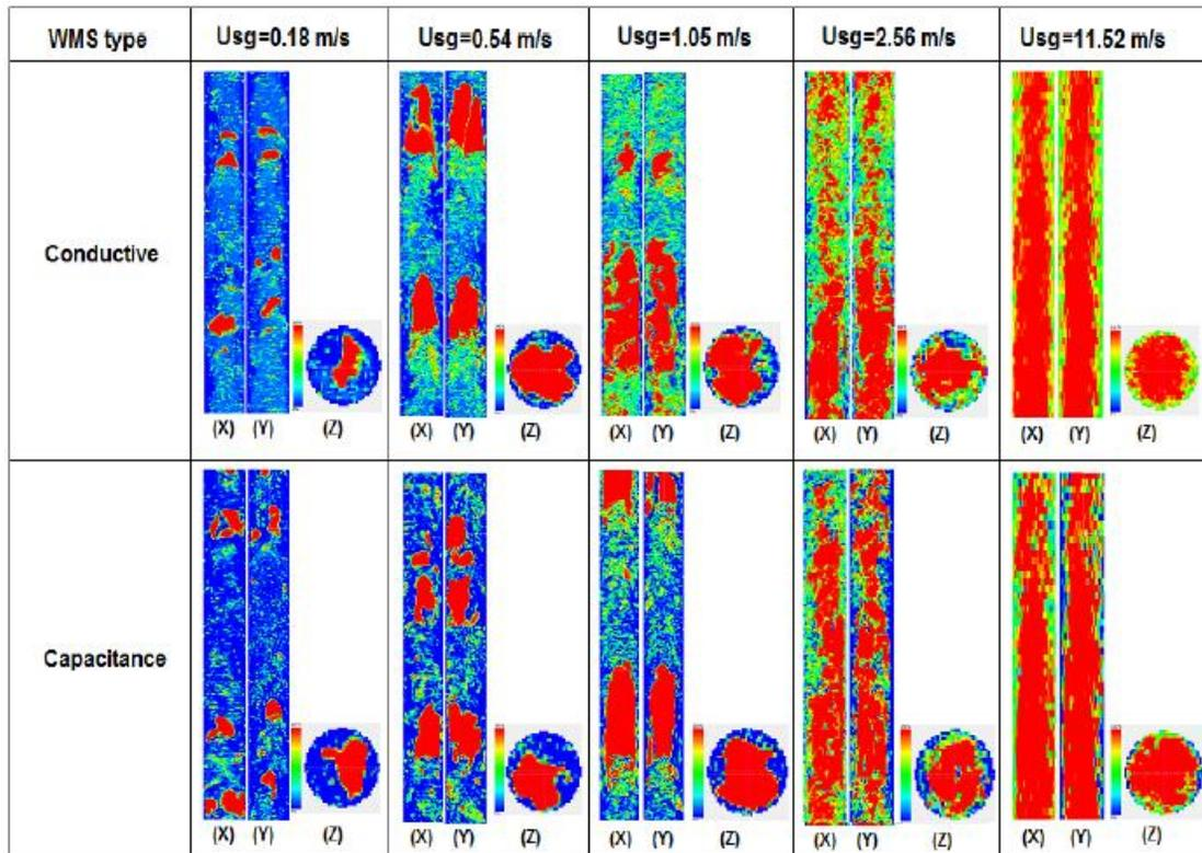
Figure 7: Reconstructed images generated by CondWMS and CapWMS at the higher location of upward orientation (X and Y depict an axially sliced images, and Z depict cross-sectional images)
