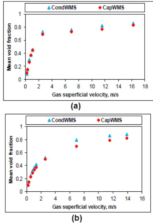
Figure 3: behavior of the void fraction against gas velocities at (a) the lower downward section and (b) the higher upward section
