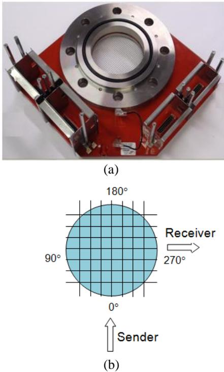
Figure 2: (a) wire-mesh sensor and (b) the two sets of wire electrodes
