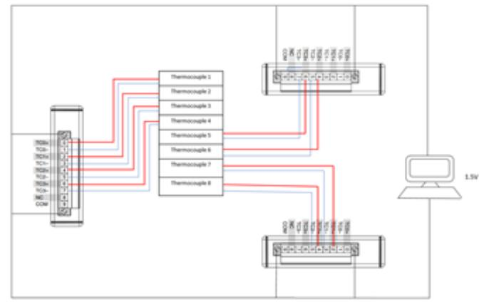
Figure 2: Thermocouple Dataq Electric Circuit
