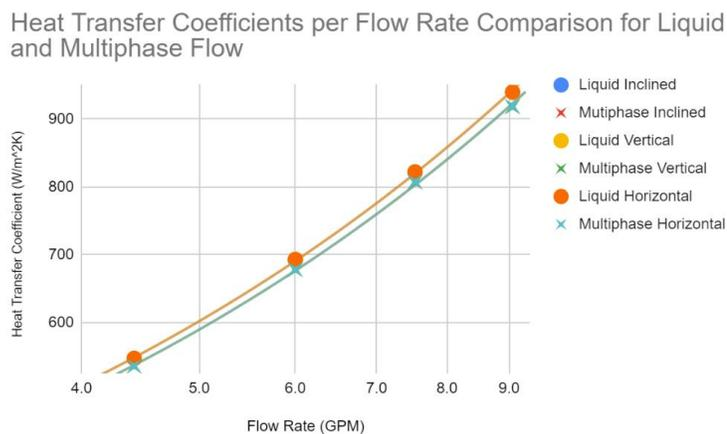
**Figure 10:** Comparison of Heat Transfer Coefficients for Liquid and Liquid/Air Flow
