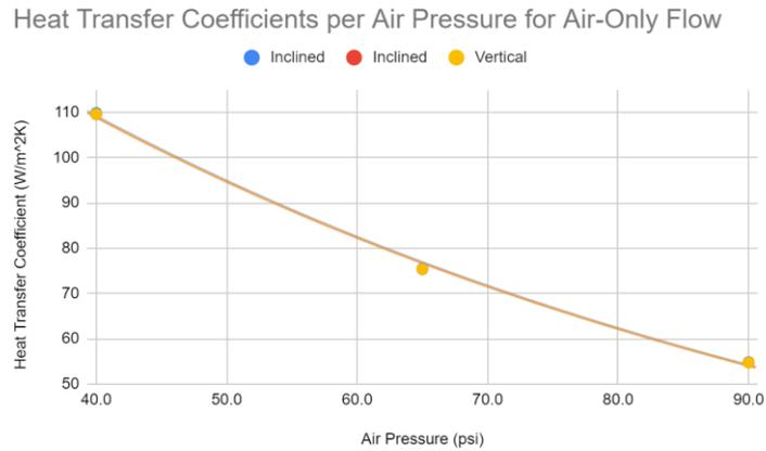
**Figure 11:** Comparison of Heat Transfer Coefficients for Different Air Pressures
