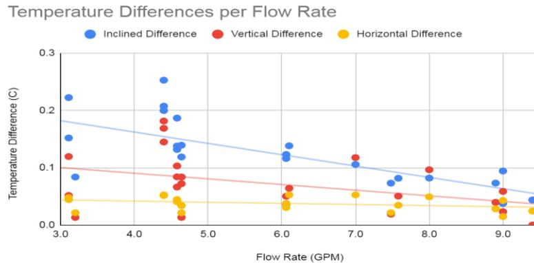
Figure 4: Temperature Difference Per Flow Rate
