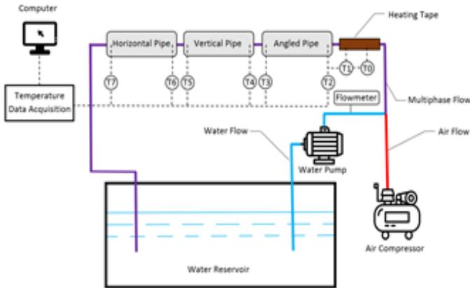
Figure 1: Thermocouple Dataq Flow Circuit
