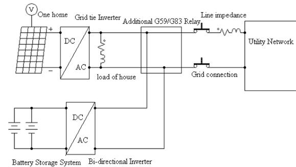
Fig. 1. Circuit diagram of the AC-Mini-Grid system
