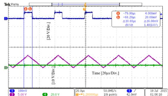
Fig. 5. The performance of the control circuit, trace 3 and trace 4 are the triangular signal and error signal respectively and trace 1 is generated PWM waveform
