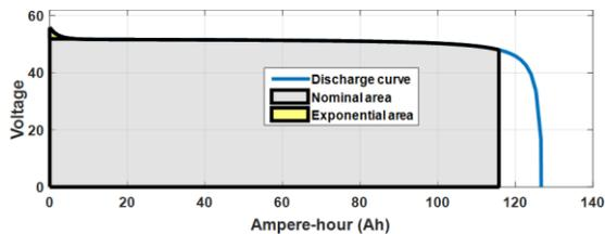
Fig. 2. Cut-off voltages for a typical battery
