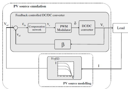
Fig. 3. Block diagram of a PV array emulator [26]
