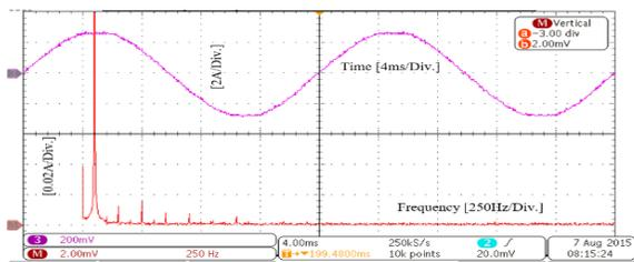
Fig. 10. Output current [10A/Div.] of the Mini-Grid goes to the domestic load and THD=0.64%
