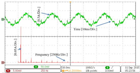
**Fig. 7.** Output current waveform of the SB700 inverter [10A/Div.] when connected to the PVAE and its FFT analysis, along with the THD which was found to be 24%
