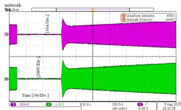
Fig. 12. Response of the AC Mini-Grid when transferring from on-grid to off-grid: trace 4 is the output voltage [200V/Div.], trace 3 is the output current [10A/Div.]
