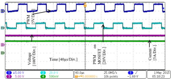
Fig. 4. Experimental measurements of the buck converter at input voltage=300V [24]
