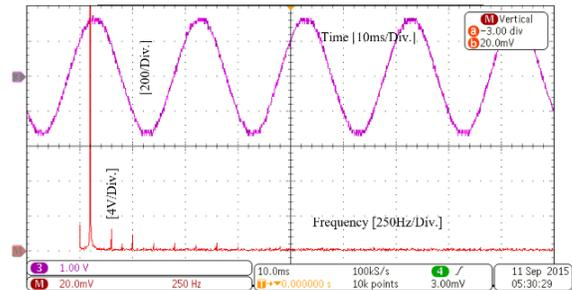
**Fig. 8:** Output voltage waveform of the SB700 inverter [200V/Div.] when connected to the PVAE and its FFT analysis, along with the THD which was found to be 4.5%
