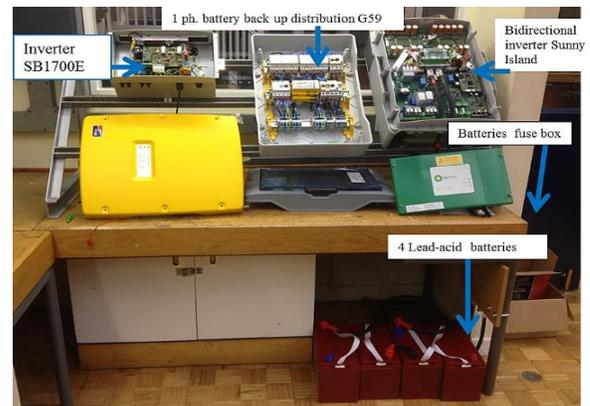
**Fig. 9.** Batteries located under the AC Mini-Grid system.
