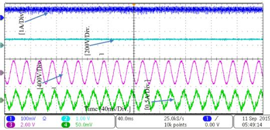
**Fig. 6.** Testing the SB700 inverter with the PVAE: trace 1 is the input current [10A/Div.], trace 2 is the input voltage [200V/Div.], trace 3 is the output voltage [200V/Div.], and trace 4 is the output current [10A/Div.]
