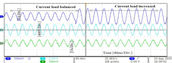
Fig. 11. Trace 1 is the output current of the AC Mini-Grid going to the resistive load [10A/Div.], trace 2 is the output voltage of the AC Mini-Grid [200V/Div.], and trace 4 is the current generated from the solar system [10A/Div.]
