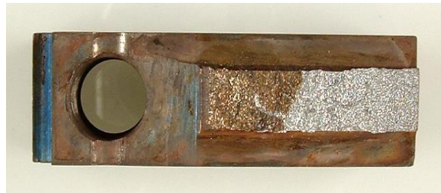
Figure 4. SCC crack forking observed for observed Karrest .
