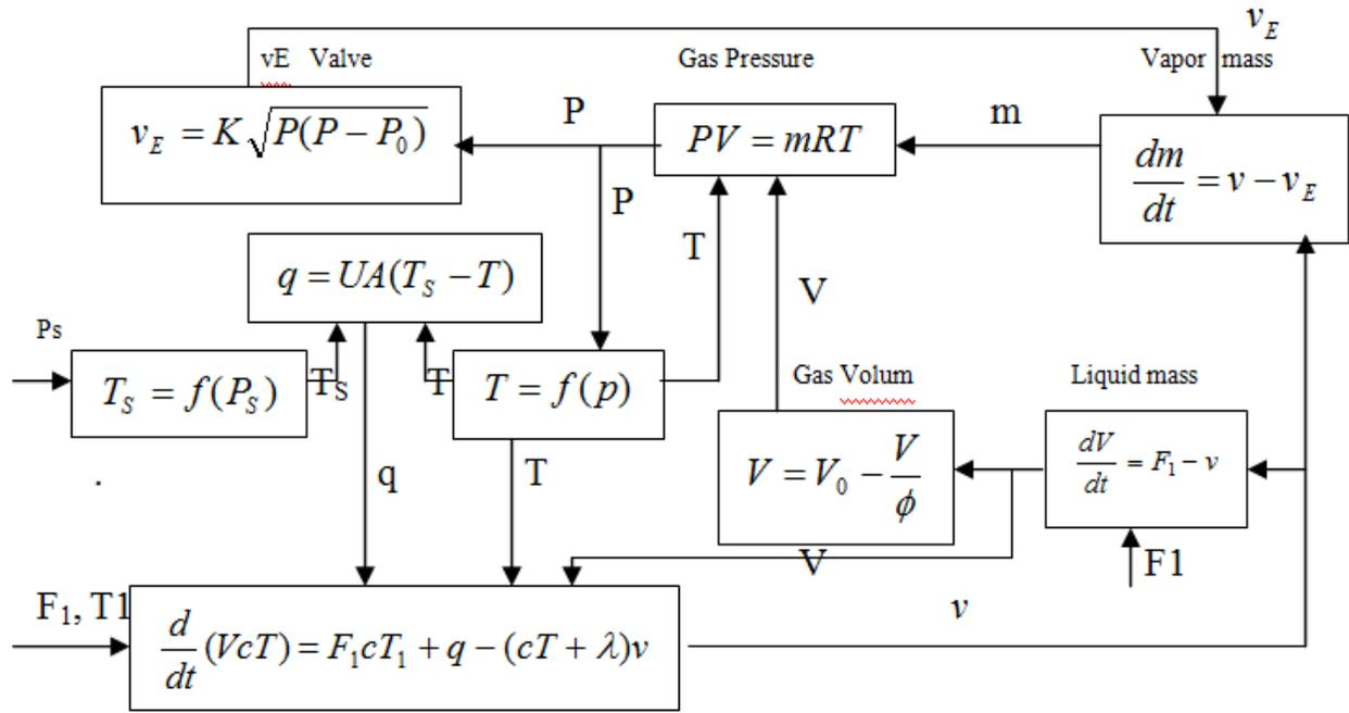
**Figure 2-1.** Model for continuous flow Boiling system.
