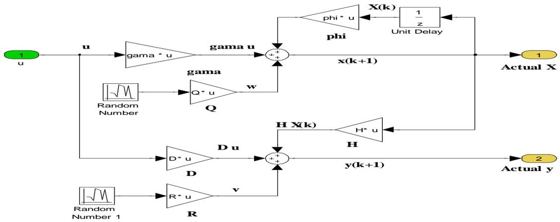
The simulink model of the Plant Equations
