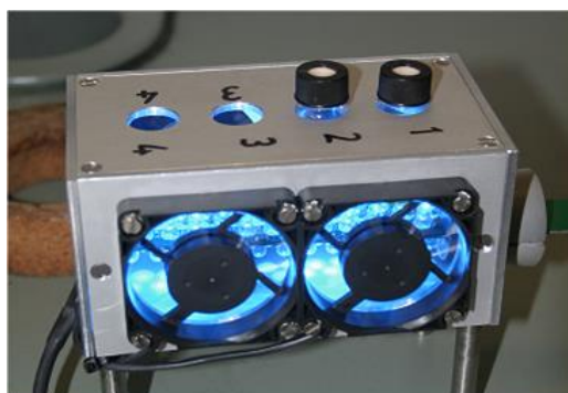
Figure 6. shows the reactor where the catalytic solutions were irradiated by blue LEDs (470 nm wavelength).
