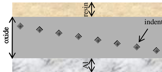
Figure (1). Schematic diagram of the indents utilized to determine the hardness on a cross-section of a porous anodic alumina film by micro-hardness technique.
