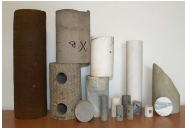
Figure (3). Full diameter core (left) and core plugs (right) cut for laboratory measurements
