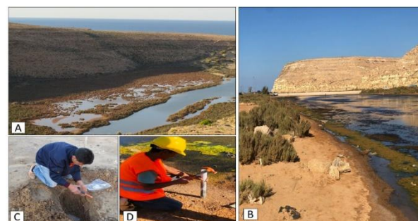
Figure. 2. A. Represents the Wadi El-Sahal sabkha. B. Shows the Wadi El-Suwani sabkha. Image C Illustrates the process of direct sample collection using the trench method where samples are placed in plastic bags. D. Shows the placement of the core sampler in the Wadi El-Suwani sabkha to preserve the samples inside the cores
