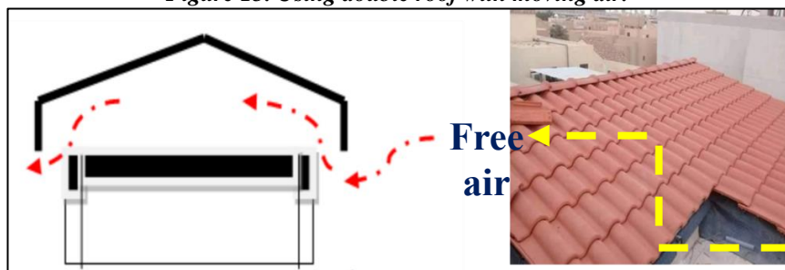
Figure 13. Using double roof with moving air.
