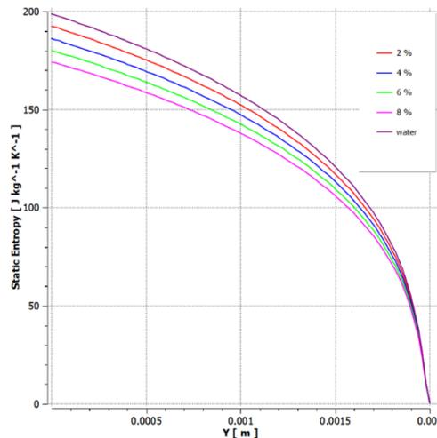
Figure 7 Entropy variation with the volume fraction along the microchannel
