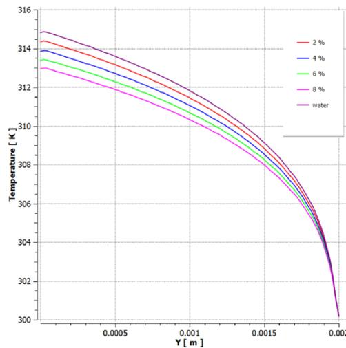
Figure 5 Variation of temperature with volume fraction along the microchannel
