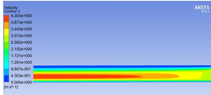
Figure 8 Velocity contour in a middle plane along the microchannel
