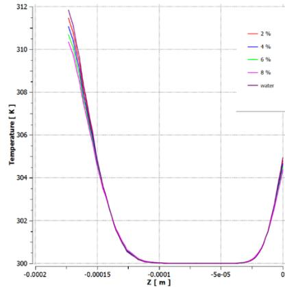
Figure 6 Variation of temperature with volume fraction on a vertical line in the middle of microchannel
