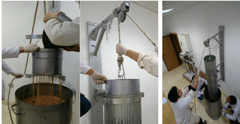
Figure 2: Compaction Testing Process Lab work
