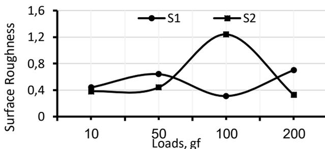
Figure 3: Surface roughness versus loads of samples.
