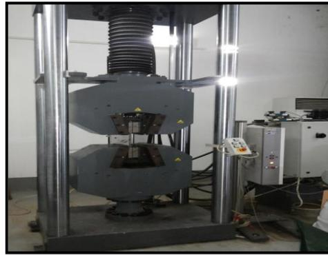
**Fig. 3: Photographic view of universal testing machine**
