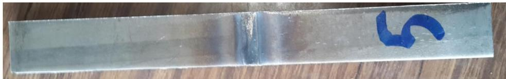
Fig. 2. Photographic view of the welded tensile test specimen
