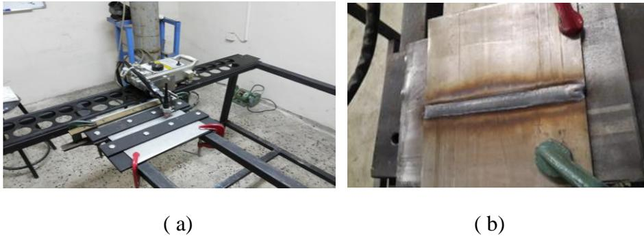
Fig. 1. a- Welding fixture and equipment setup, b- Butt joint of DSS-2205
