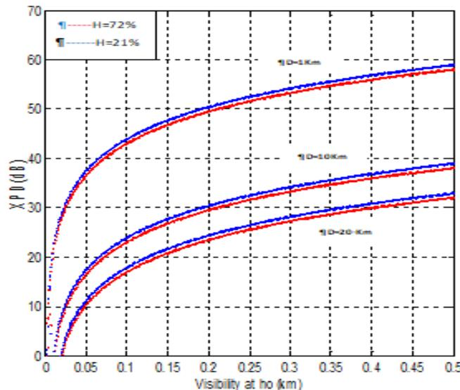
**Figure.5. Cross Polarization Discrimination (dB) at height= 10m.**
