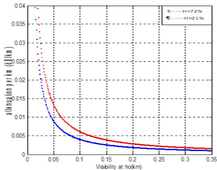
**Figure.3 Attenuation per km at height= 10m and for for two types of dust.**
