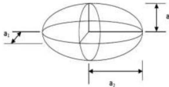
**Figure 1 Dust Particle Geometry Approximation.**
