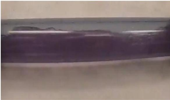
**Figure 10:** Stratified Wavy Flow
