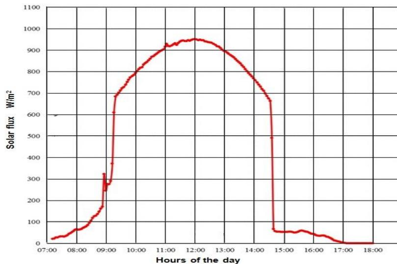
Fig. 5 Variation of solar flux using Immhx2 on October 31
