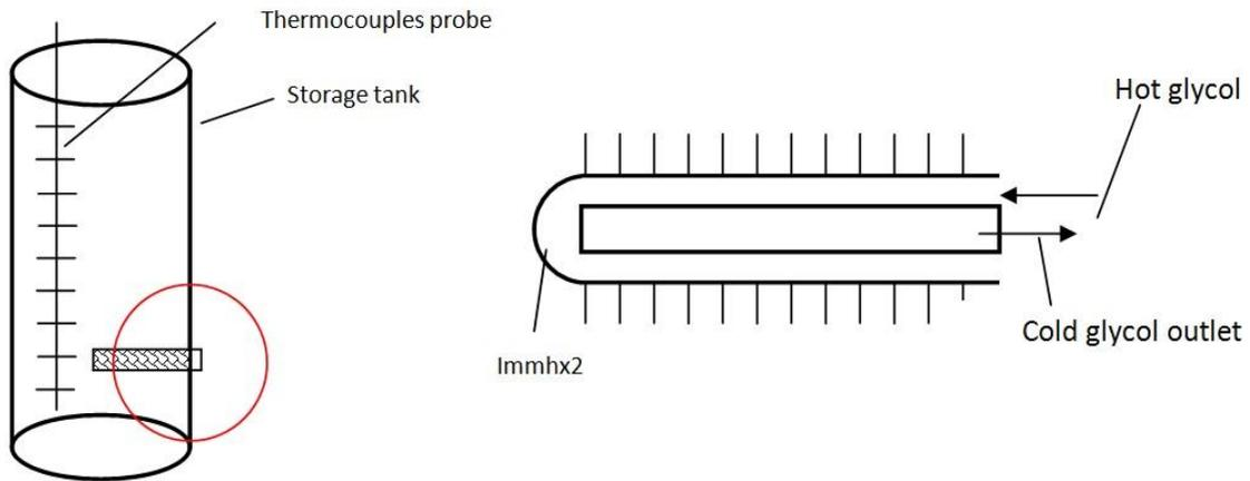
Fig. 3 Schematic diagram of second immersion heat exchanger (Immhx2)
