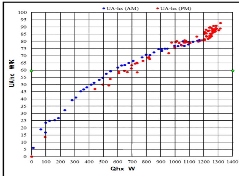
Figure 6 Heat transfer coefficients (UA), the heat transfer rate (qhx) of ImmS&Chx on October 21
