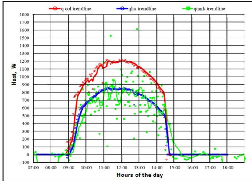
Fig. 11 Variation of heat transfer with the time on October 31 using Immhx2
