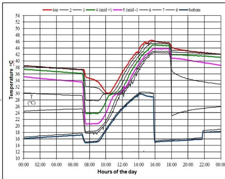
Fig. 8 The temperature distribution in the storage tank for the Immhx1
