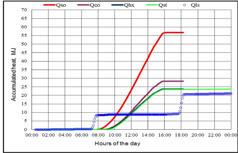
Fig. 12 Variation of accumulated heat with on October 21 using Immhx1
