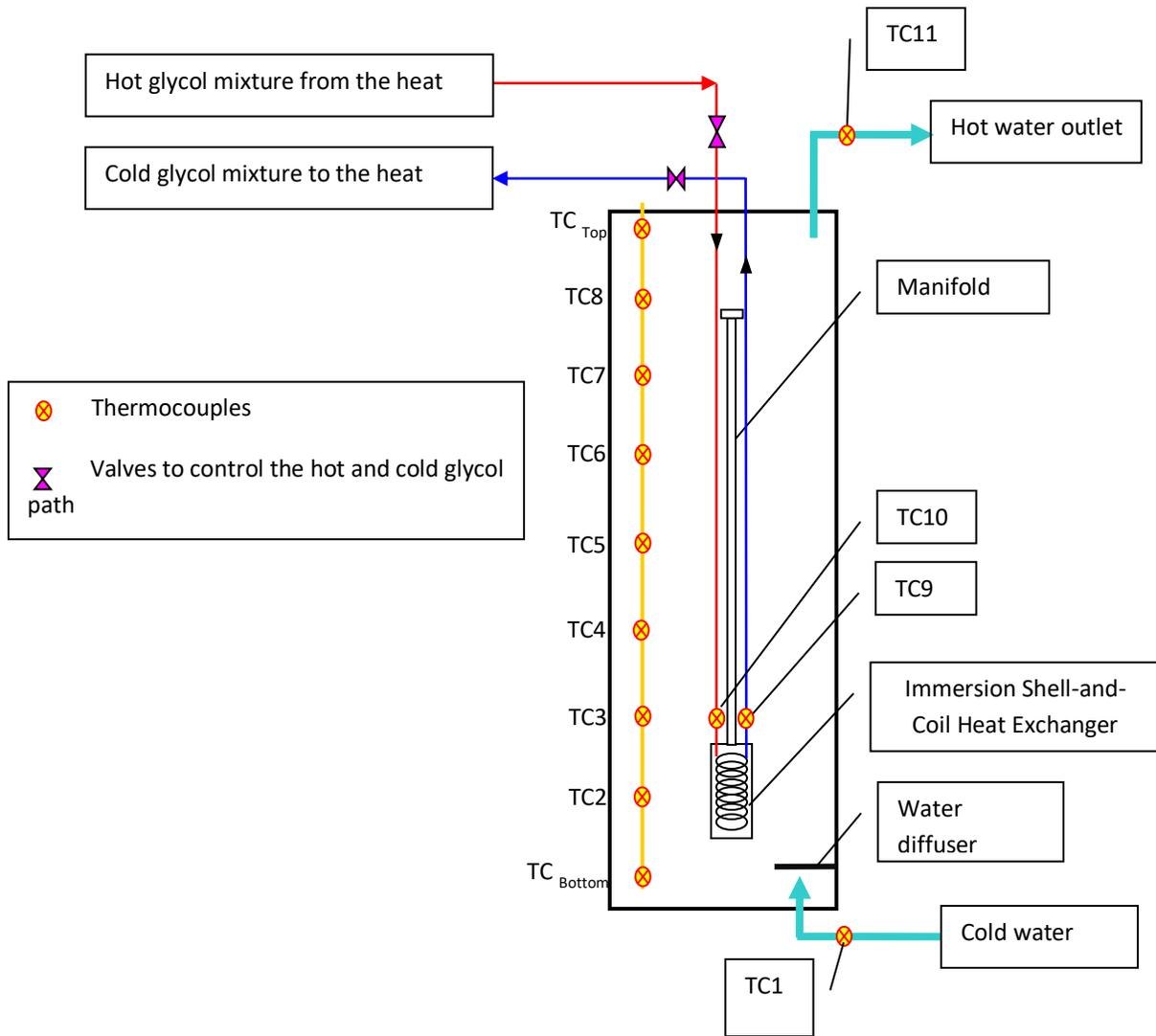
Fig. 2 schematic diagram of first immersion heat exchanger (Immhx1)
