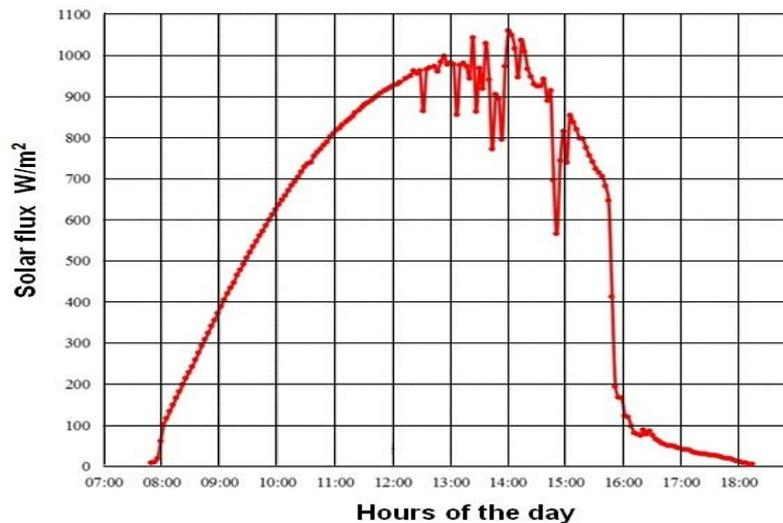
Fig. 4 Variation of solar flux using ImmS&Chx on October 21
