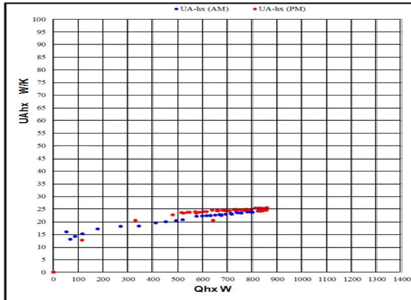
Figure 7 Heat transfer coefficients (UA) Vs. the heat transfer rate (qhx) of Immhx2
