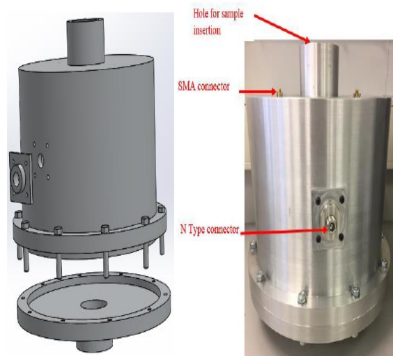
Figure 1 large aluminum cylindrical cavity resonator. [9]
