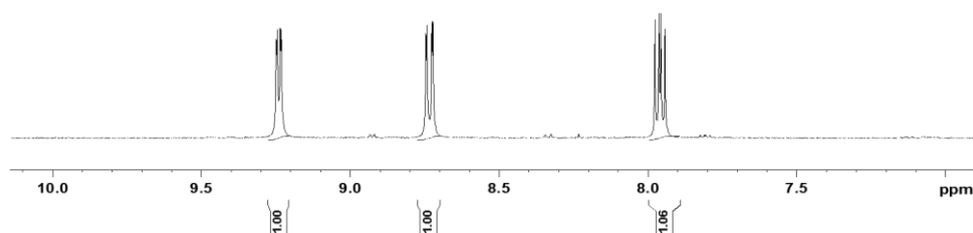
**Figure 10:**  $^1\text{H}$  NMR spectrum for 1,10-phenanthroline-5,6-dione,  $[\text{Re}(\text{CO})_3(1,10\text{-phenanthroline})\text{Cl}]$  and  $[\text{Re}(\text{CO})_3(1,10\text{-phenanthroline-5,6-dione})\text{Cl}]$  in  $\text{d}_6\text{-Acetone}$  at 298K.
