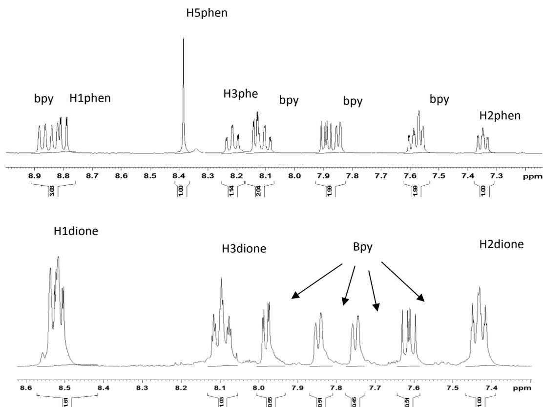
**Figure 8:** <sup>1</sup>H NMR spectrum for [Ru(bpy)<sub>2</sub>(1,10-phenanthroline)]<sup>2+</sup> and [Ru(bpy)<sub>2</sub>(1,10-phenanthroline-5,6-dione)]<sup>2+</sup> in d<sub>3</sub>-Acetonitrile at 298K.
