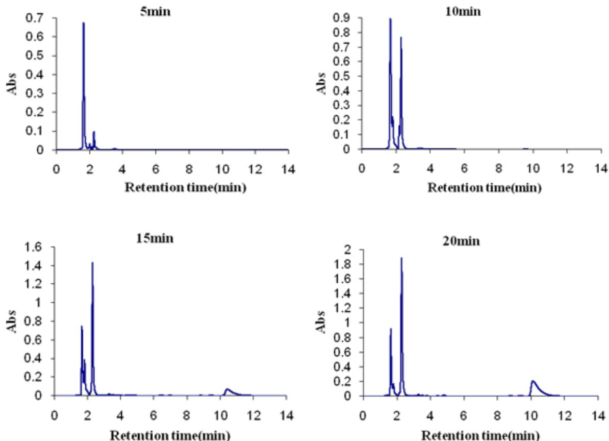
**Figure 13:** HPLC trace for [Ru-Ru](a) , [{Ru-Re}(b) , [{Re-Re}(c) and photolysis of [Ru-Ru](d) in CH<sub>3</sub>CN (mobile phase CH<sub>3</sub>CN: H<sub>2</sub>O with volume ratio 80:20 containing 0.1 M KNO<sub>3</sub>). Flow rate: 2.0 cm<sup>3</sup> min<sup>-1</sup>; detection wavelength at 280 nm.
