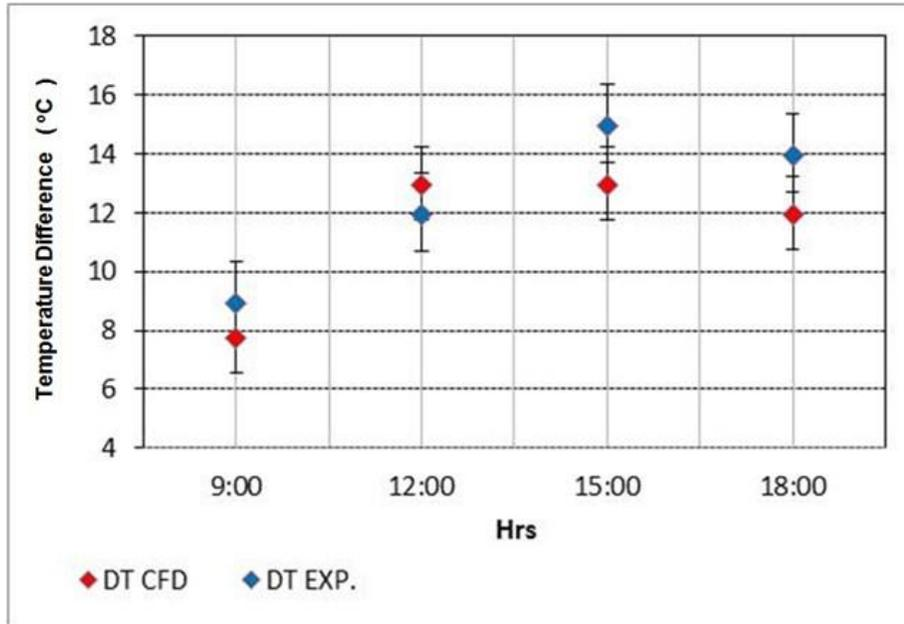
Figure 11 Comparison of experimental and CFD results of temperatures difference between outdoor and indoor environments of office
