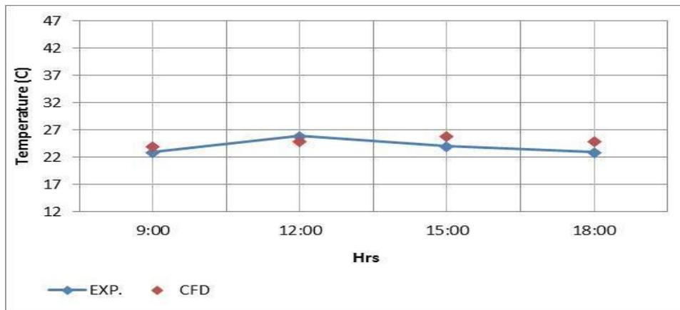
Figure 9. Comparison of variation of internal temperature with time for experimental and CFD results
