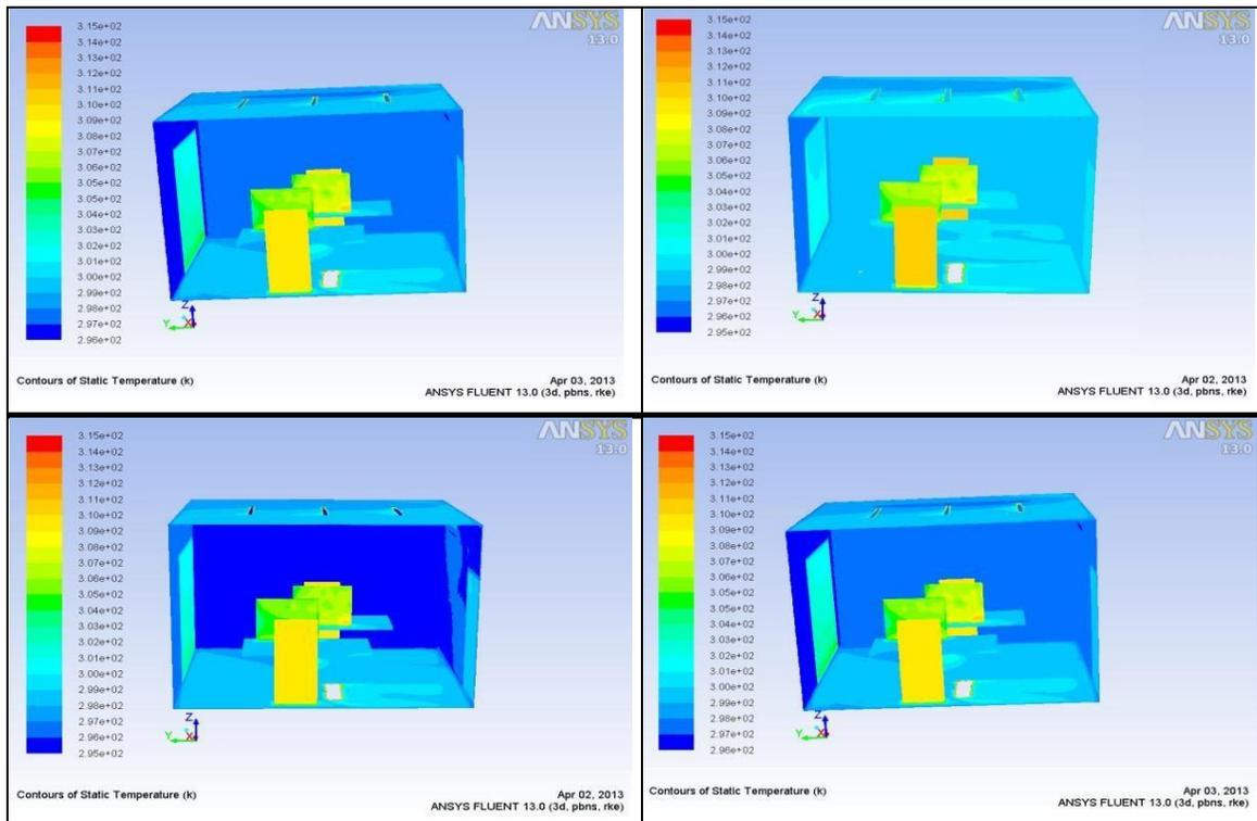
Figure 5. The average temperature distribution in the office using CFD simulation
