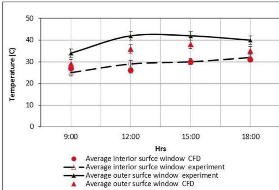
Figure 10. Comparison of experimental and CFD results of inner and outer glass surfaces
