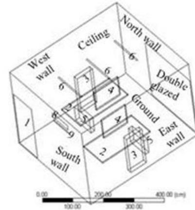
Figure 3. Surface boundary condition of test office
