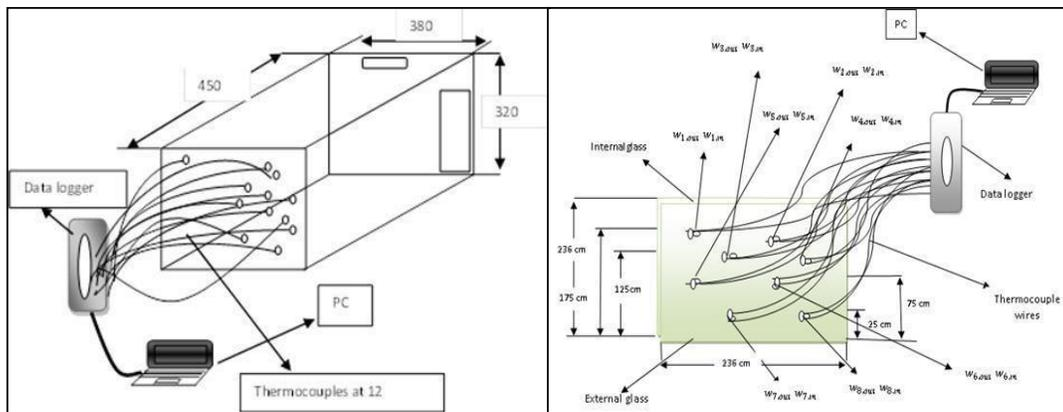
Figure 8. Thermocouples locations in the office and above external and internal surfaces of double-glazed window
