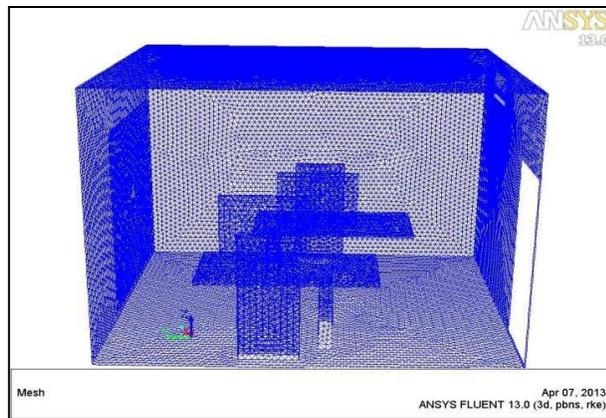
Figure 4. Grid mesh generation
