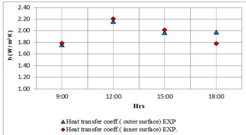
Figure 14. Comparison of experimental results of inner & outer surface heat transfer coefficient
