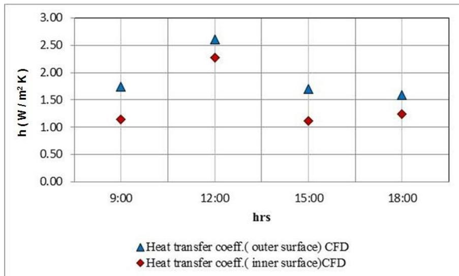
Figure 15. Comparison of CFD results of inner & outer surface heat transfer coefficient
