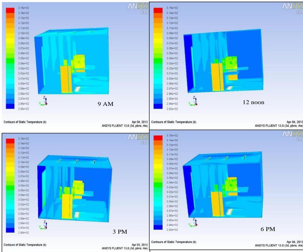
Figure 6. Temperature distribution inside the room at different time
