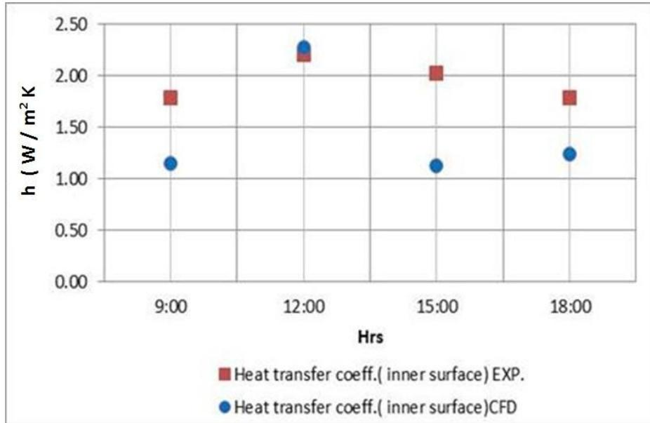
Figure 12. Variation of experimental and CFD of heat transfer coefficient (inner surface ) with time
