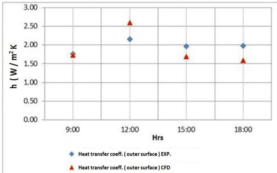
Figure 13. Variation of Experimental and CFD Heat Transfer Coefficient (Outer Surface) with Time
