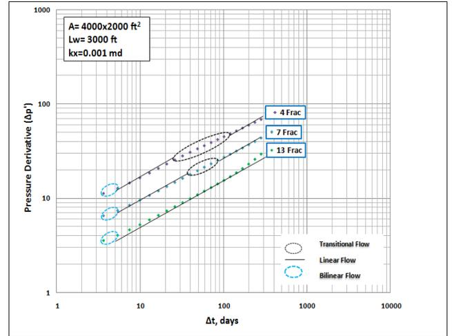
**Figure 6 -7.** The impact of the number of hydraulic fractures ( $w_f= 0.1$  inch)
