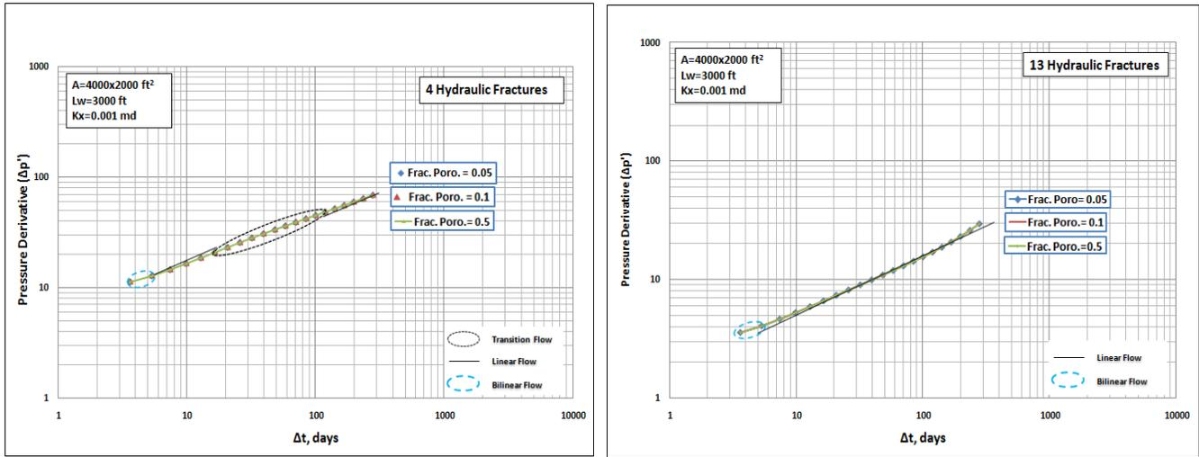
**Figure 22-23.** The impact of fracture porosity on hydraulic fractures
