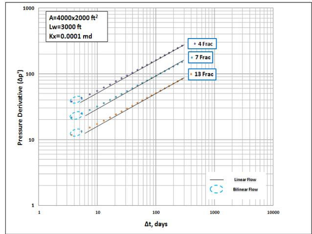
**Figure 12-13.** The impact of fracture width ( $w_f=0.01$  inch)
