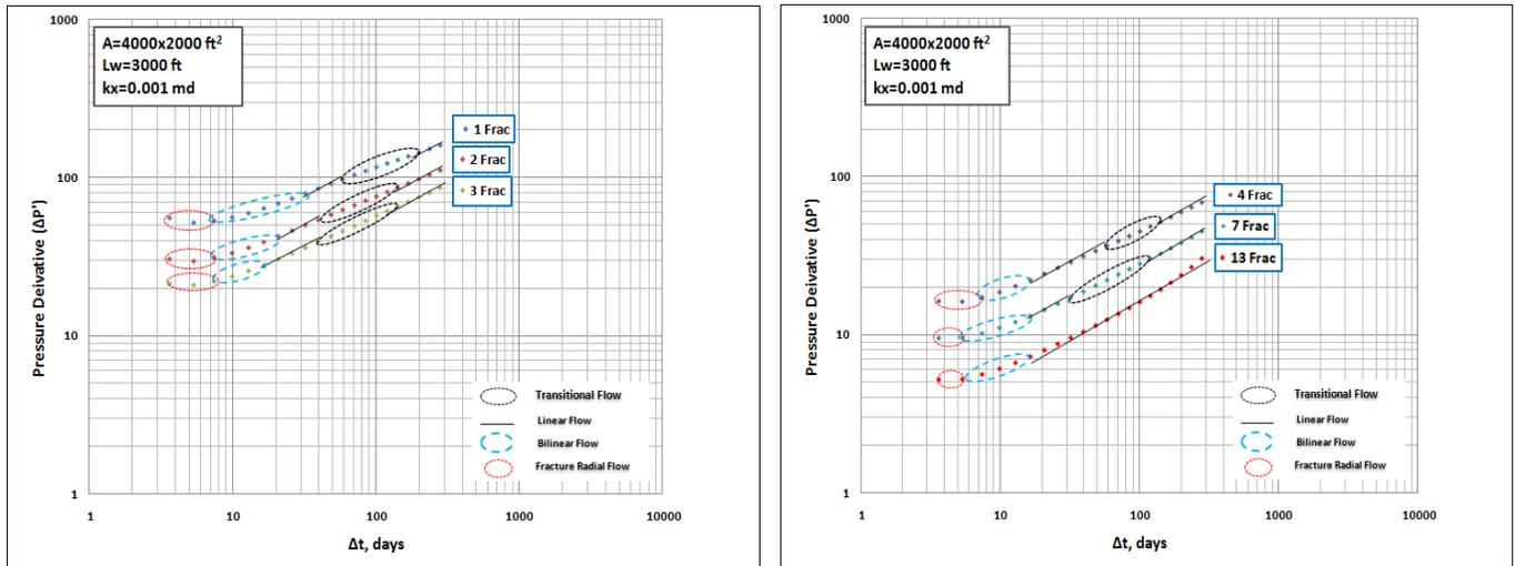
**Figure 10-11. The impact of fracture width ( $w_f= 0.01$ inch)**
