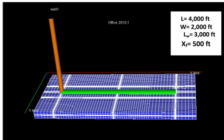
**Figure 3.** A horizontal well model with a 4,000 ft by 2,000 ft and well length of 3,000 ft.
