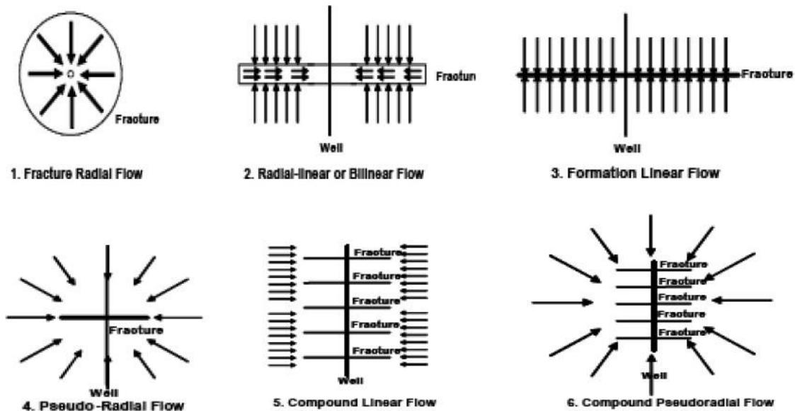
**Figure 1.** Flow regimes for fractured horizontal wells [6]
