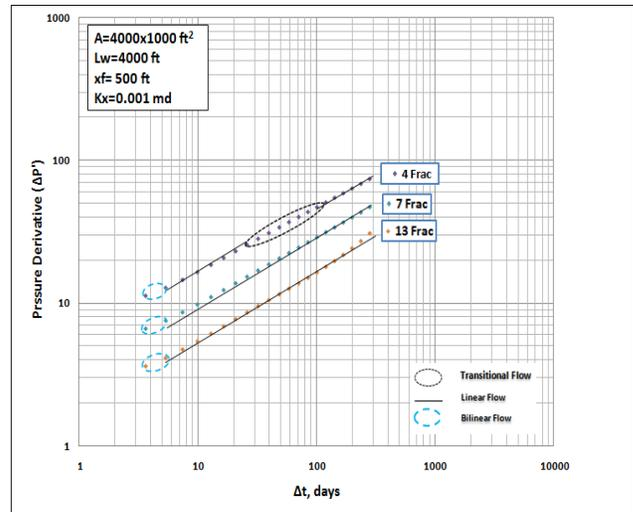
**Figure 14-15.** The impact of drainage area and horizontal well length ( $w_f=0.1$  inch)
