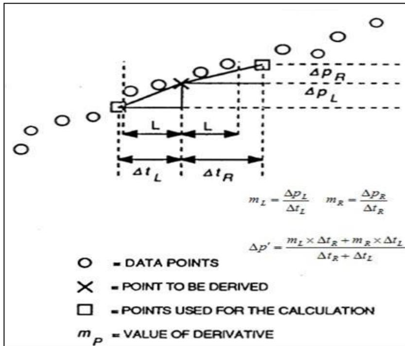
**Figure 5.** Five-point method for calculating the pressure derivative [4].
