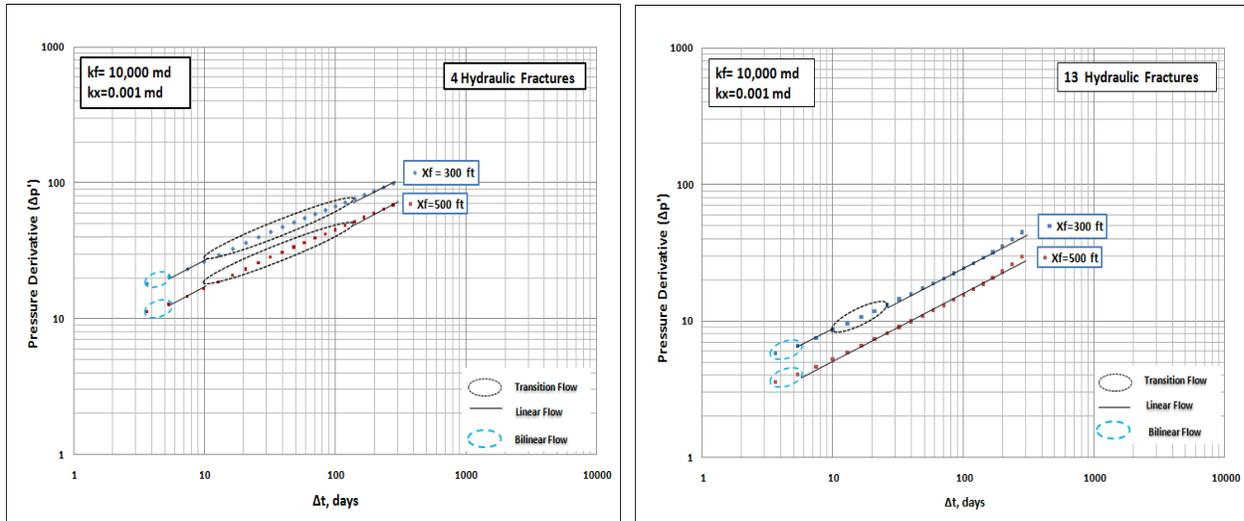
**Figure 20-21.** The impact of fracture half-length on hydraulic fractures
