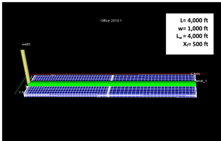
**Figure 4.** A horizontal well model with 4,000 ft by 1000 ft and well length of 4,000 ft
