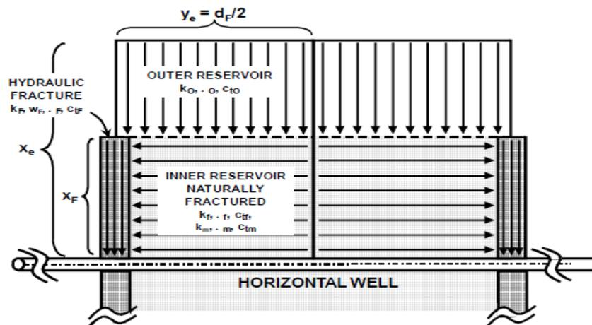
Figure 2. Trilinear flow regimes for multiple fractured horizontal well [5]
