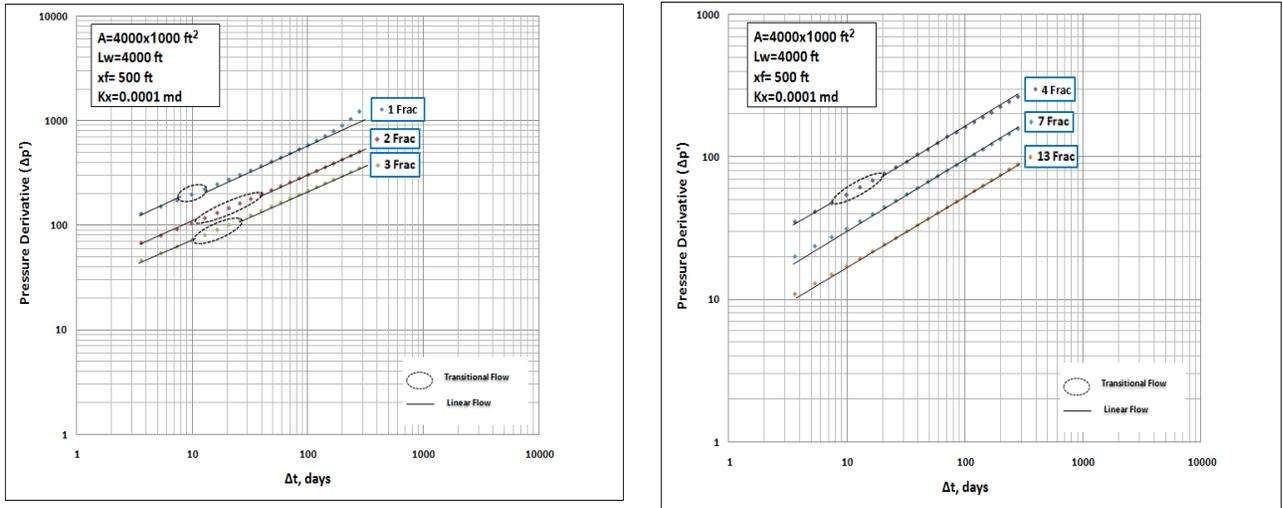
**Figure 16-17.** The impact of drainage area and horizontal well length ( $w_f=0.1$  inch)
