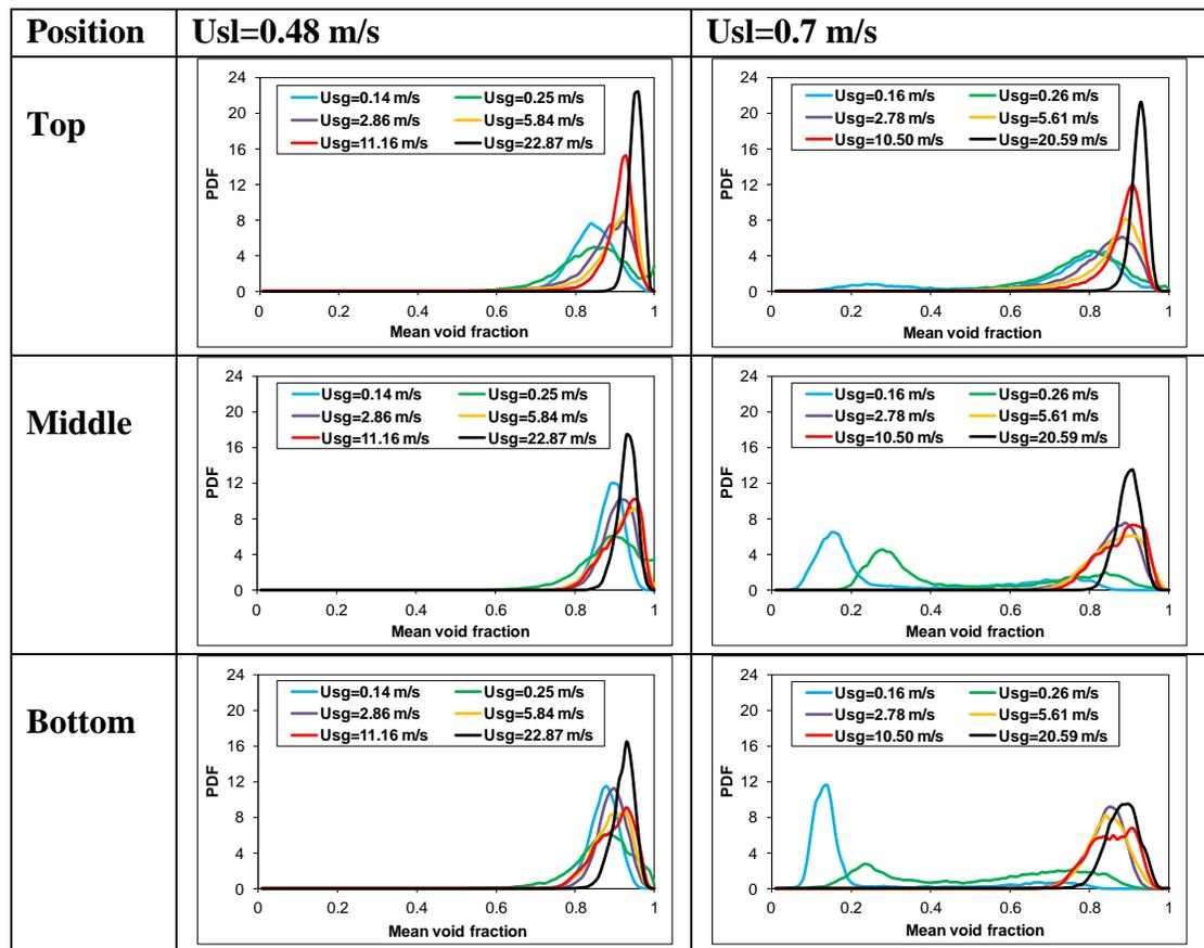
Figure 5 PDFs of the average void fraction at the top, middle and bottom positions of downward section
