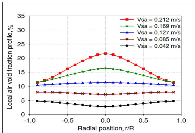
Figure 3 Local distribution of gas void fraction obtained from ERT for liquid superficial velocity of 1.039 m/s (Olni et al., 2013)
