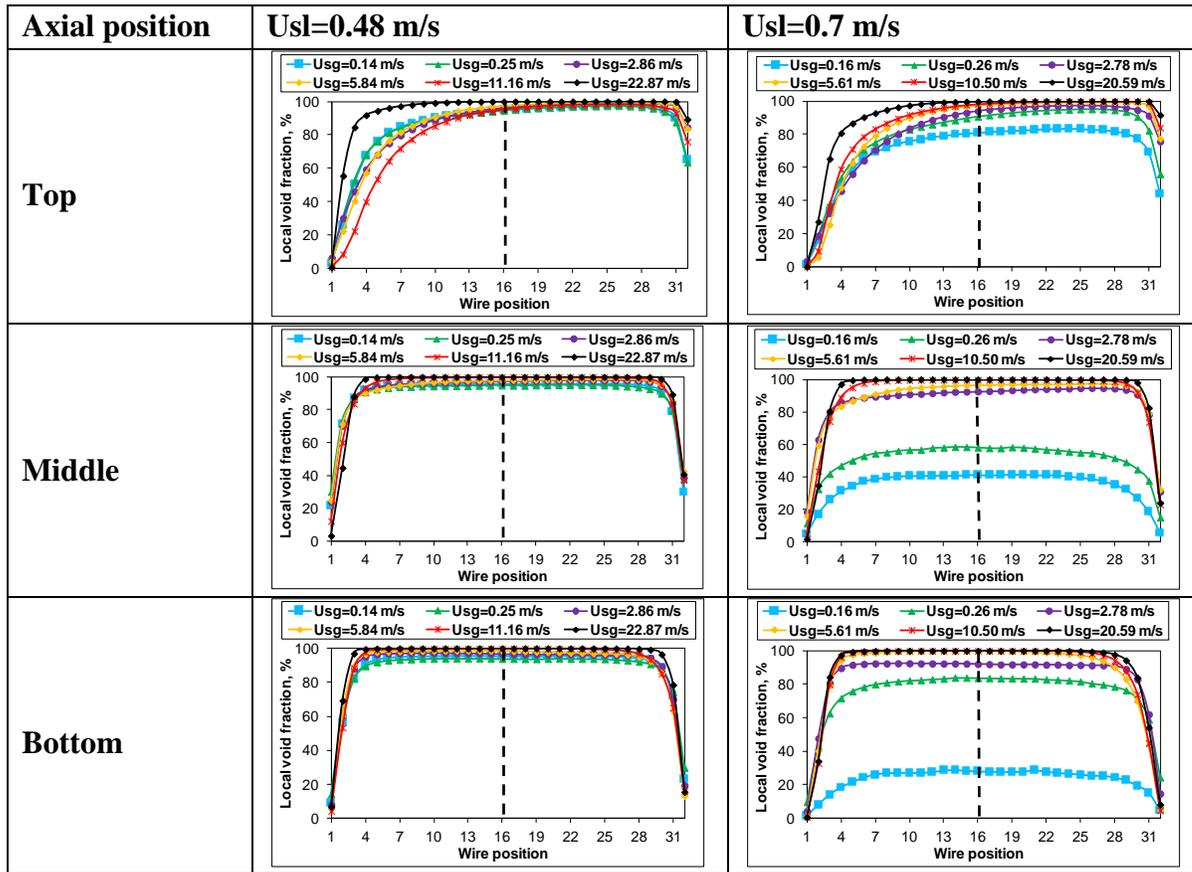
Figure 6 Local void fraction distribution from 90 to 270° measured at the top, middle and bottom positions of downward section
