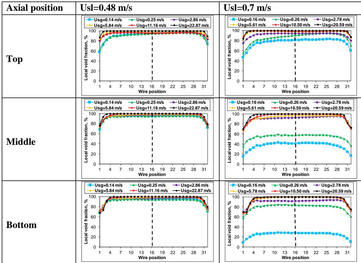
Figure 7 Local void fraction distribution from 0 to 180° measured at the top, middle and bottom positions of downward section
