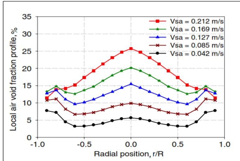
Figure 2. Local distribution of gas void fraction obtained from WMS for liquid superficial velocity of 1.039 m/s (Olni et al., 2013)
