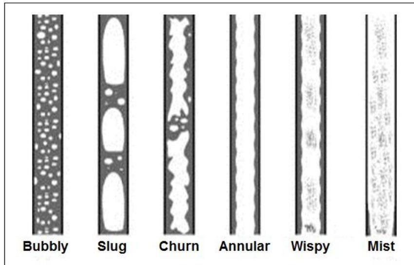
Figure 1 Gas-liquid flow patterns in vertical pipes (Cheng et al., 2008)
