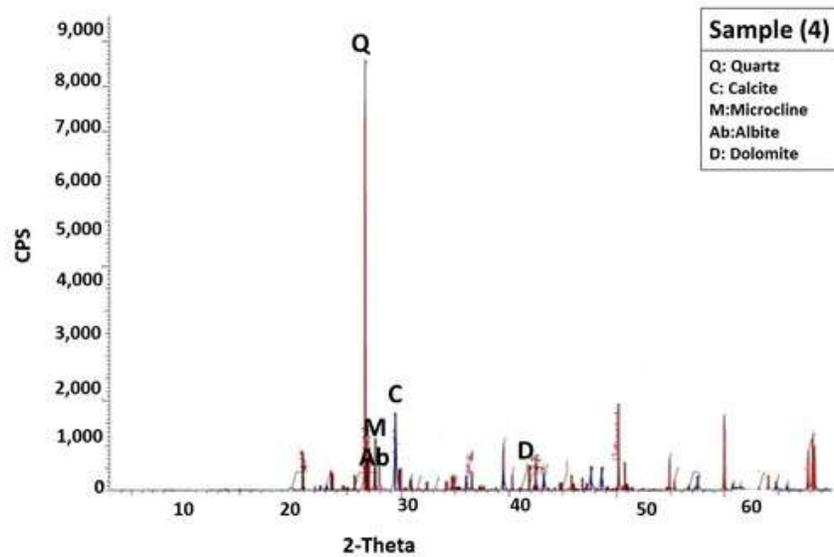
Fig.11. Typical X-ray diffraction pattern showing the total mineral components identified in Al-Suwani Supratidal sabkha.
