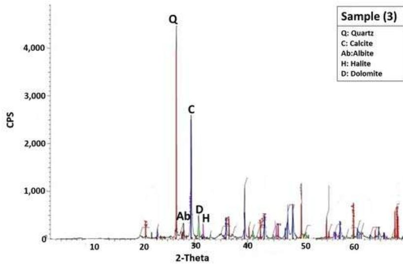
Fig.10. A typical X-ray diffraction pattern shows the total mineral components identified in Al-Suwani intertidal sabkha.
