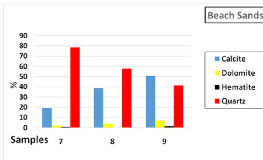
Fig. 18. Bar graph representation showing the relative percentages of the bulk minerals in the Beach sand sediments.
