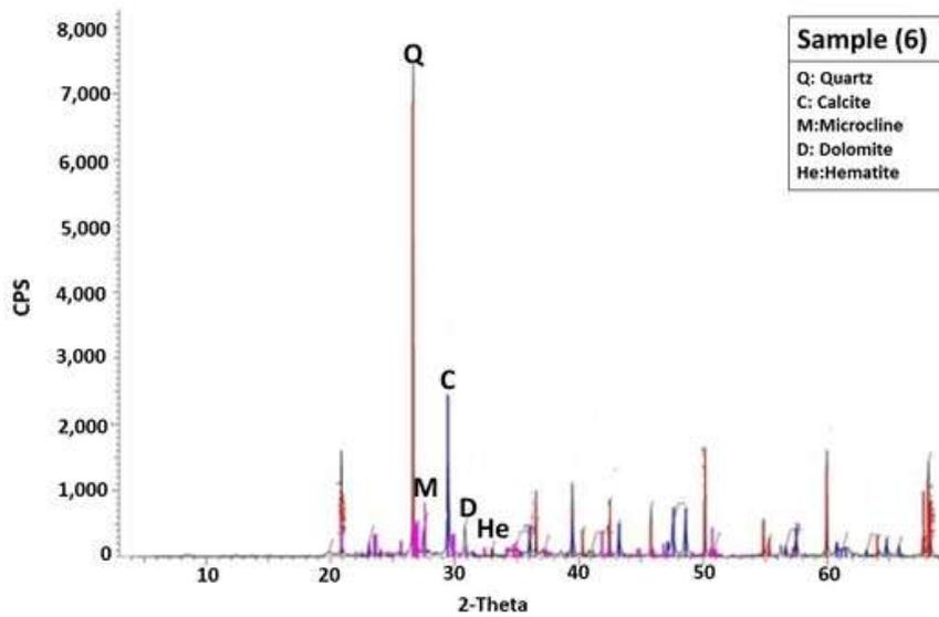
Fig.13. Typical X-ray diffraction pattern showing the total mineral components identified in Al-Suwani Supratidal sabkha.
