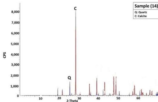
Fig. 23. X-ray diffraction pattern showing the bulk mineral components identified in rock cliffs of Al Faidiyah Formation.
