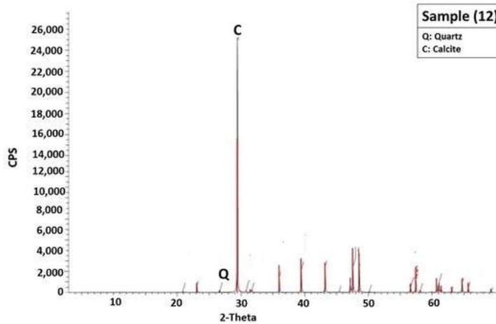
Fig. 21. X-ray diffraction pattern showing the bulk mineral components identified in rock cliffs of Al Jaghubub Formation.
