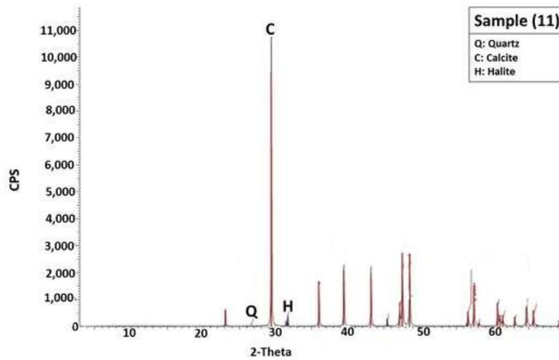
Fig.20. X-ray diffraction pattern showing the bulk mineral components identified in rock cliffs of Al Faidiyah Formation.
