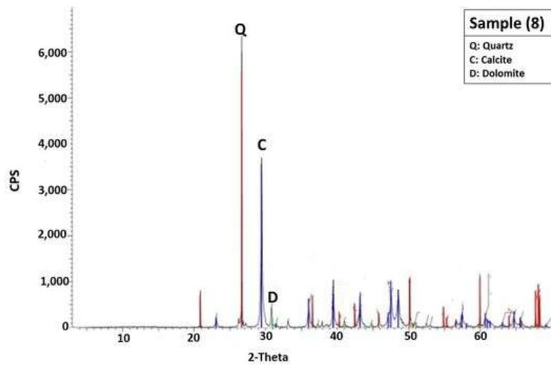
Fig. 16. A typical X-ray diffraction pattern shows the total mineral components identified in Beach sand
