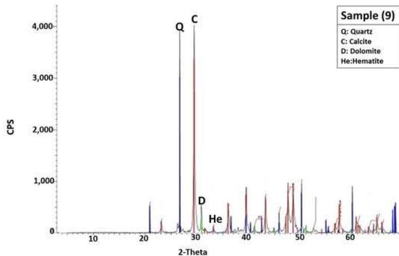
Fig. 17. A typical X-ray diffraction pattern showing the total mineral components identified in Beach sand.
