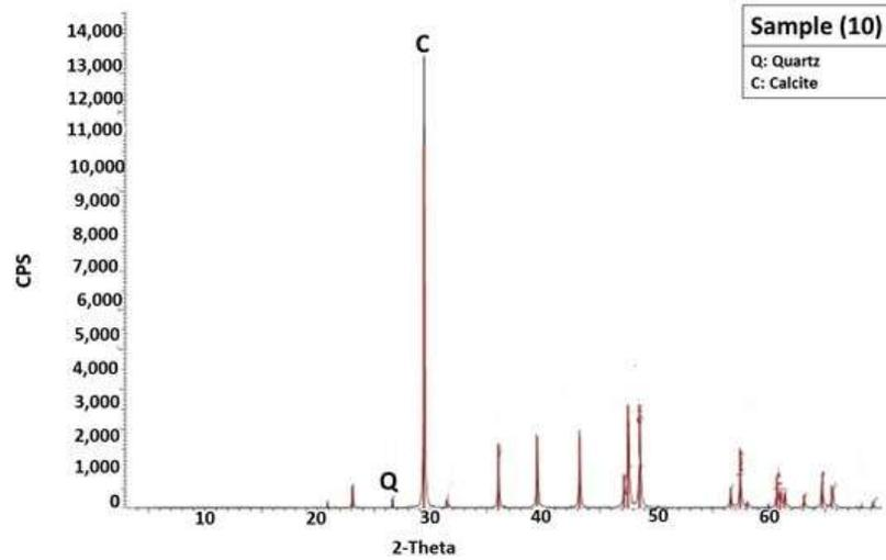
Fig. 19. X-ray diffraction pattern showing the bulk mineral components identified in rock cliffs of Al Abrag Formation.
