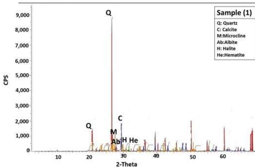
Fig.8. A typical X-ray diffraction pattern shows the total mineral components identified in Al-Suwani-intertidal sabkha.
