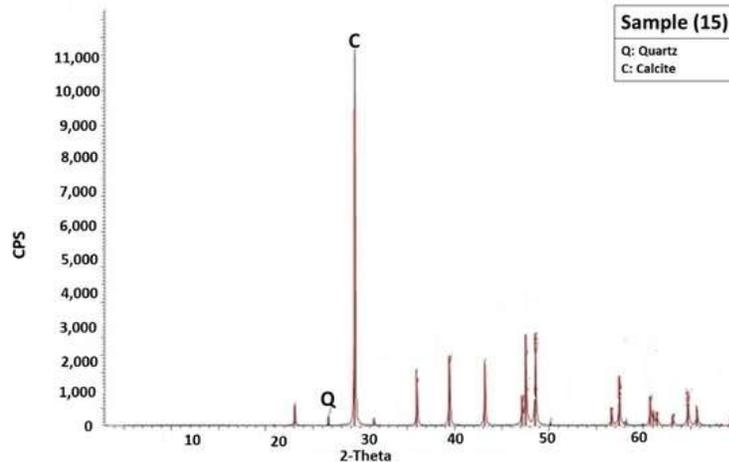
Fig. 24. X-ray diffraction pattern showing the bulk mineral components identified in rock cliffs of Al Jaghub Formation.
