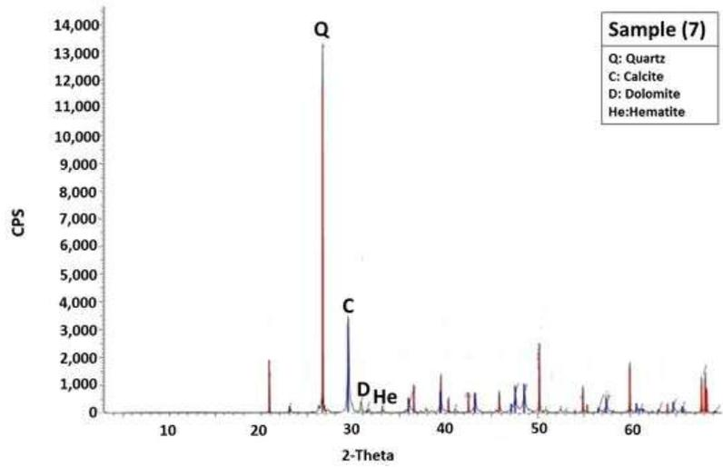
Fig. 15. A typical X-ray diffraction pattern shows the total mineral components identified in Beach sand.
