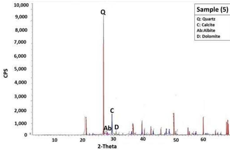
Fig.12. Typical X-ray diffraction pattern showing the total mineral components identified in Al-Suwani Supratidal sabkha.
