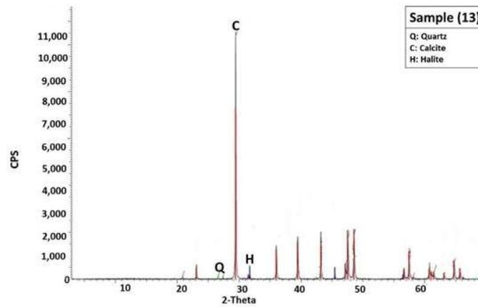
Fig. 22. X-ray diffraction pattern showing the bulk mineral components identified in rock cliffs of Al Abrag Formation.
