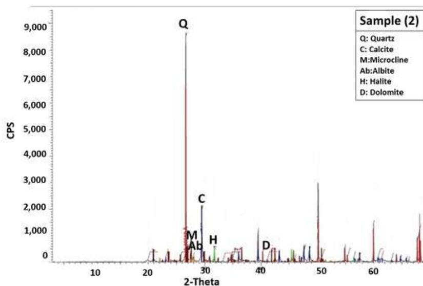
Fig. 9. A typical X-ray diffraction pattern shows the total mineral components identified in Al-Suwani intertidal sabkha.
