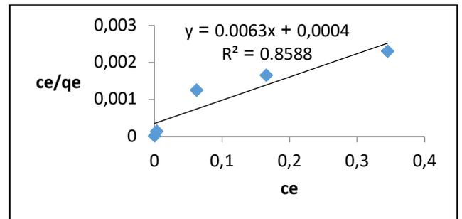
Figure 9: The Langmuir isotherm of methylene dye adsorption on (silk vine roots).
