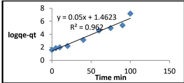
Figure 7: The first-order reaction for the adsorption process.
