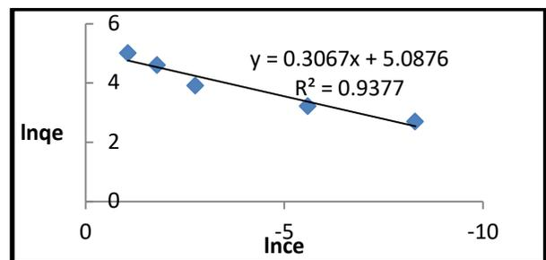
**Figure 10:** The Freundlich Isotherm of methylene dye adsorption on (silk vine roots).
