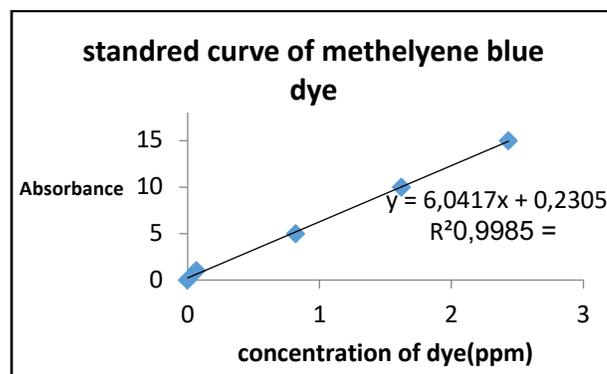
Figure 3. 1: standard curve of methylene blue dye.
