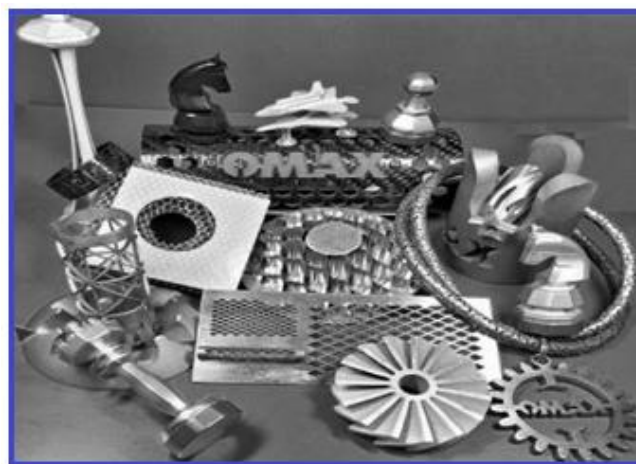
Figure 4 : Samples of AWJ machined 3D parts [6]
