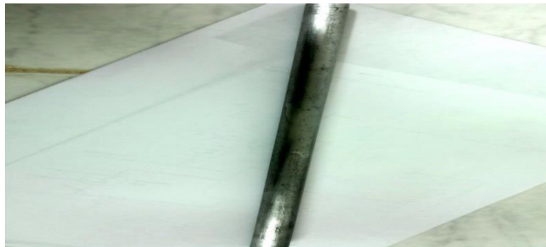
Figure. (2) The general corrosion on the test sample after immersion of 95 days in natural seawater environment and after removing all existing corrosion product and well surface cleaning.
