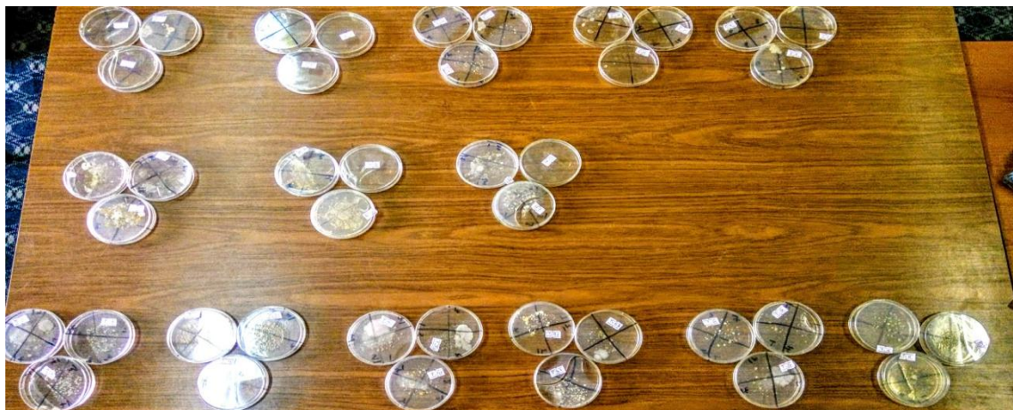
Plate 1. Plate count Agar plates for Heterotrophic Plate Count is in (cfl/mL) of the water samples
